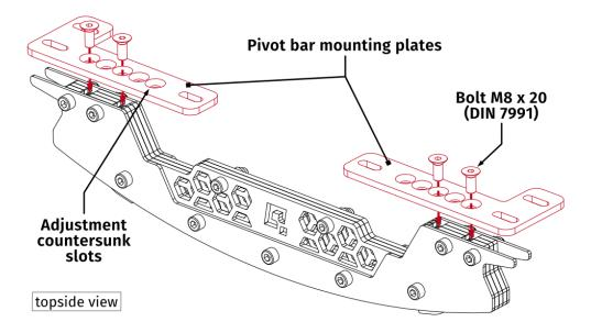
2. Screw the QS-Pivot bar in under the cockpit using included bolts.
